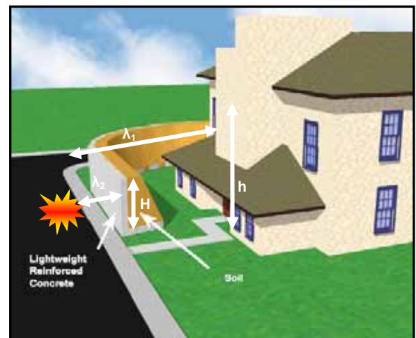
Figure 1.19 Schematic of Blast Wall and Parameters
