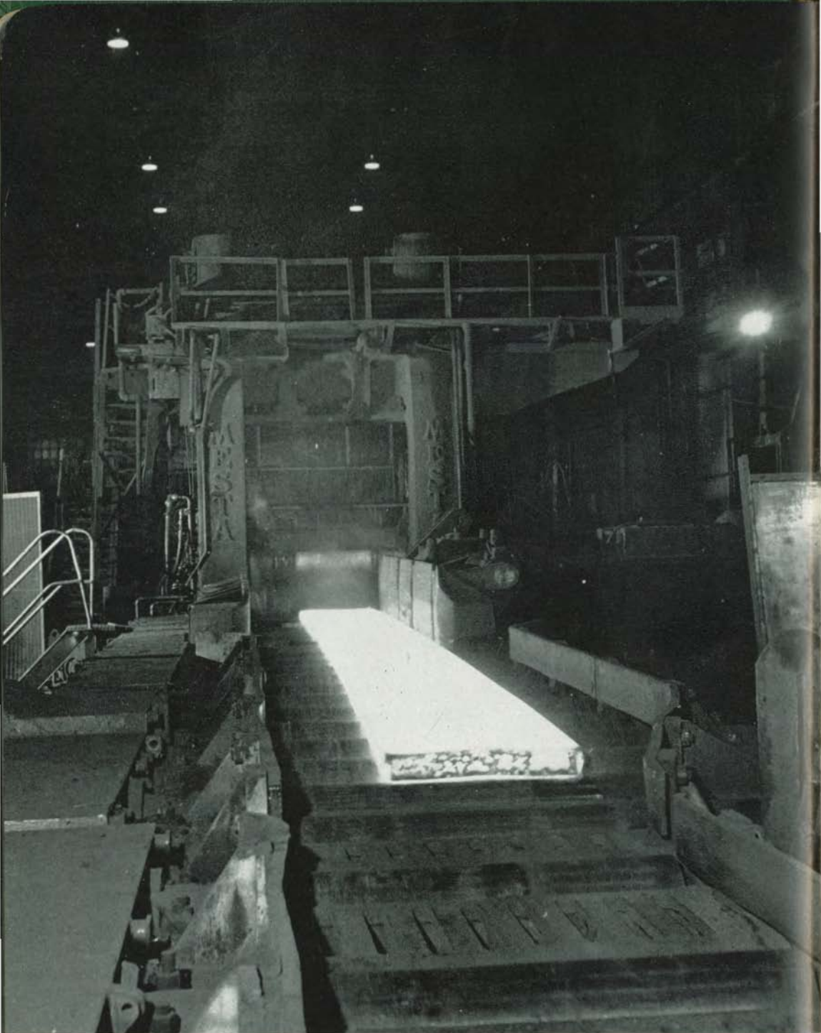
In the 36-inch blooming mill ingots are reduced to slabs and blooms. Here a slab emerges from the bloomer on its way to the plate mill.
