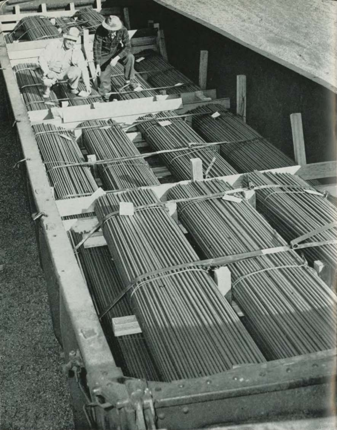
Careful loading practice insures delivery of hot rolled rods in good condition.
