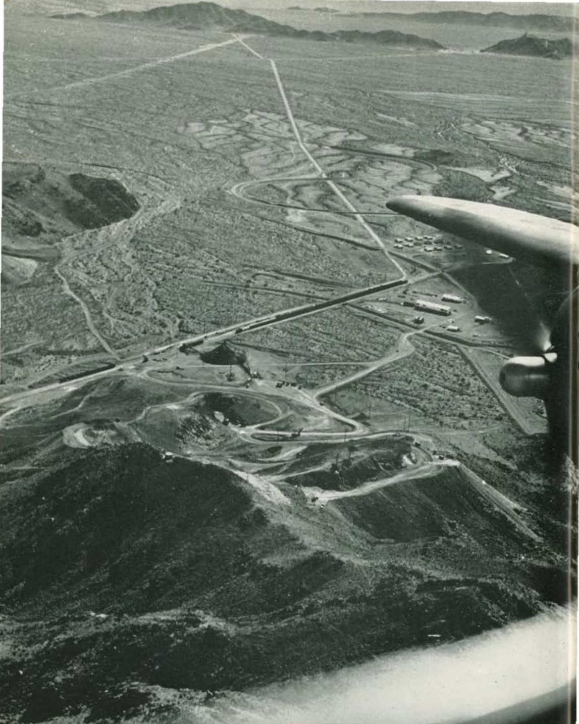
1,500,000 tons of ore, averaging 54 per cent iron content, leave Kaiser's Eagle Mountain open pit mine annually for the short 164 mile rail haul to Fontana.
