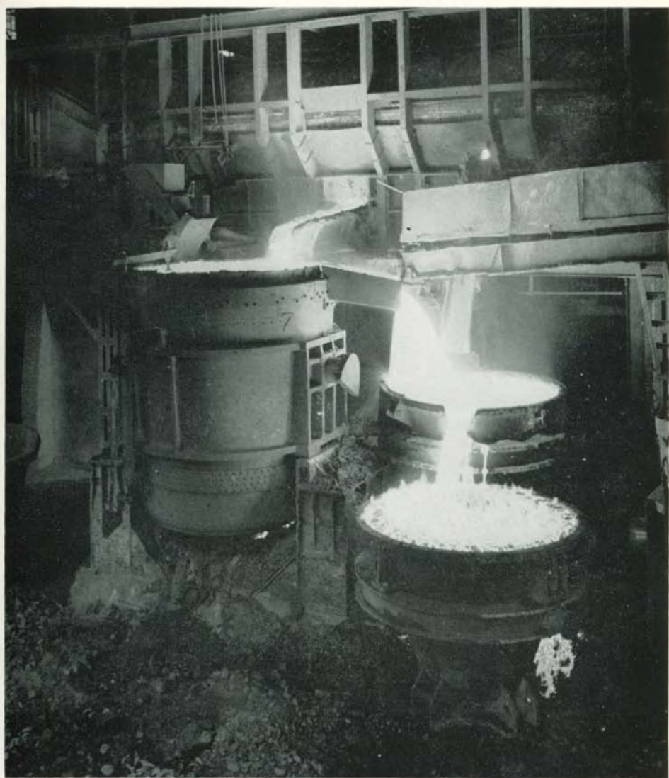
The seven open hearth furnaces at Fontana average 220 tons of steel at each tapping. The mill now is producing at the rate of 1,200,000 ingot tons per year
