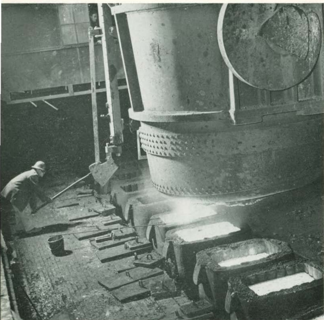
A ladleman operates a stopper rod that permits molten steel to flow through a nozzle in the bottom of the ladle into ingot molds. Ingots are poured in many shapes and sizes to meet varying rolling requirements.
