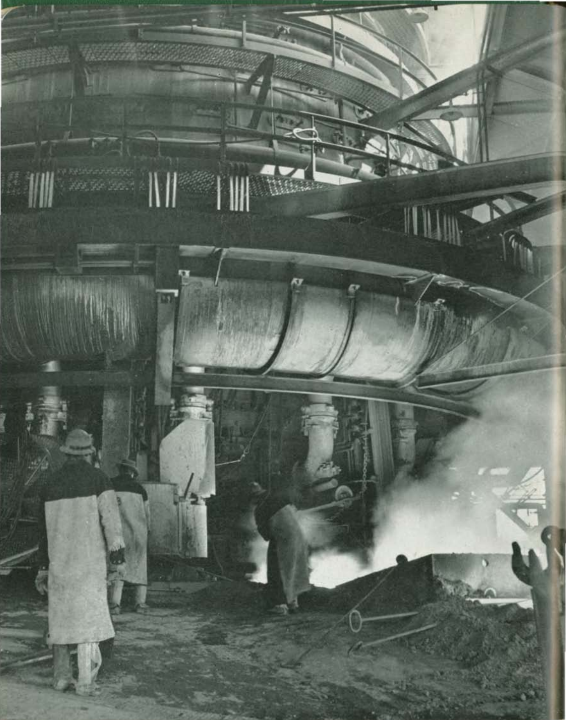
On the casting floor of a Kaiser Steel blast furnace where 250 tons of pig iron are drawn off every five hours. Two furnaces are in operation.
