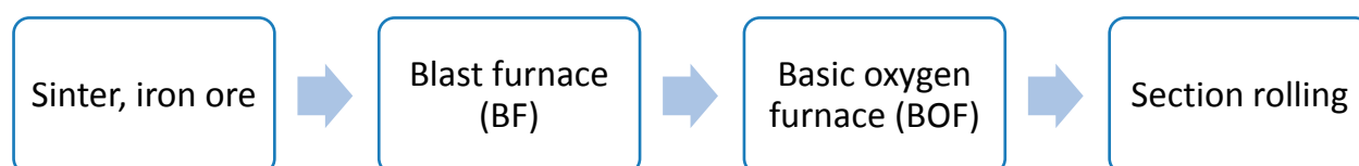
Figure 3-3: Structural section BF/BOF process flow
