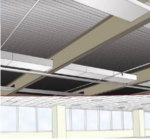
Web penetrations provide savings in floor-to-floor height.
