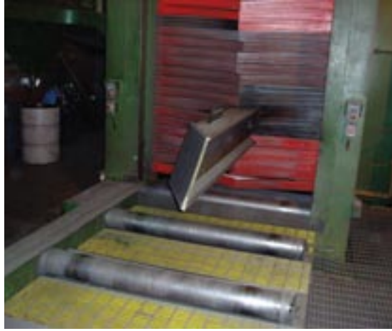
A member exits a rotary blast machine. Photo courtesy of Zimmerman Metals, Denver.
