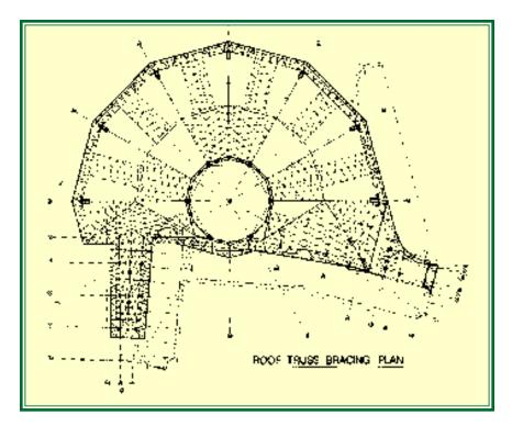
and bottom chords, and double angle web members. These trusses support conventional truss girders spaced equally between tied-arch trusses. Bar joists, approximately 26" deep, frame between the truss girders to support the skylight system.
