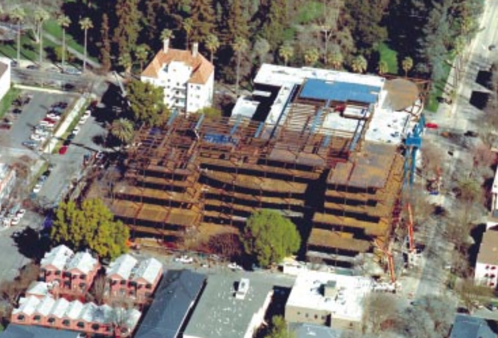
Because steel is lightweight, the structural and foundation systems are half the weight of an equivalent concrete structure.
