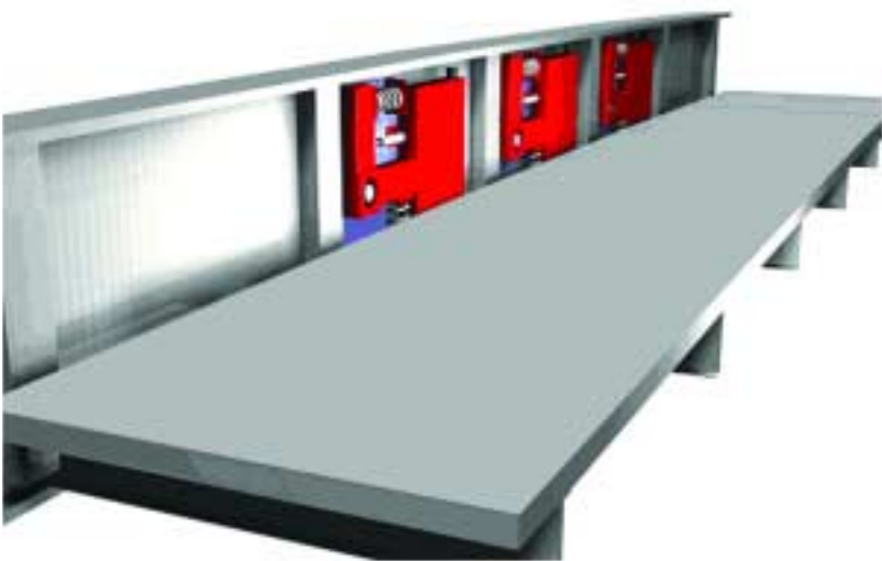
Layout of TMDs on pedestrian bridge in Las Vegas.
