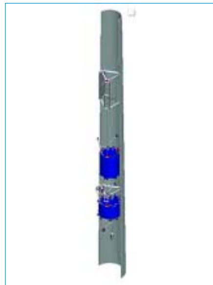
Spire Section showing tuned mass dampers.
