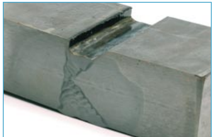
A multi-Pass weld sample (some weldments require as many as 70 passes), performed via automation.
