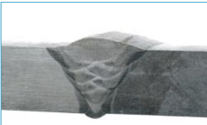
A synchronized tandem MIG multi-pass weld sample on thick weldment, performed via automation.
