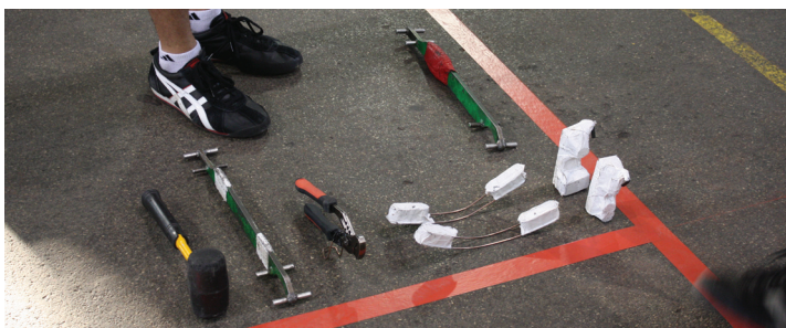
Above, below: The University of California at Davis design included several custom tools for holding members in place and making connections, shown below in the staging area and above in use during construction.
