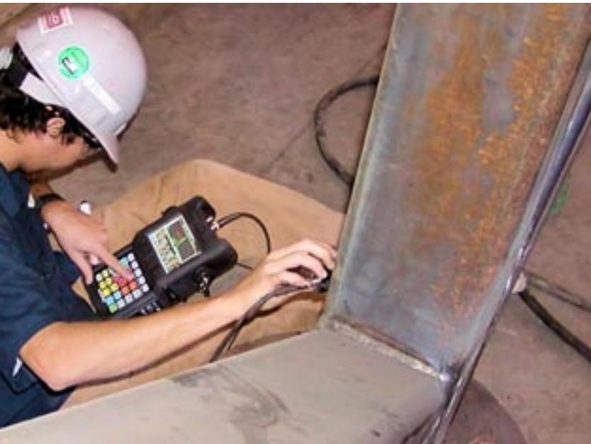
Above: Ultrasonic testing of full-penetration welds ensures they contain no inclusions or porosity and verifies that the welds are, in fact, full-penetration.
