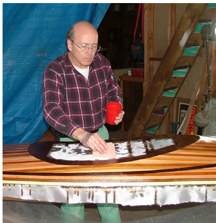
◀ Stelter applying the fiberglass to the deck of his cedar strip kayak. To see more photos, visit www.modernsteel.com/photos .
