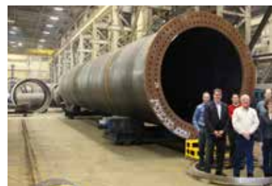
▼ The bottom two sections are straight 11-ft-diameter cylinders.
