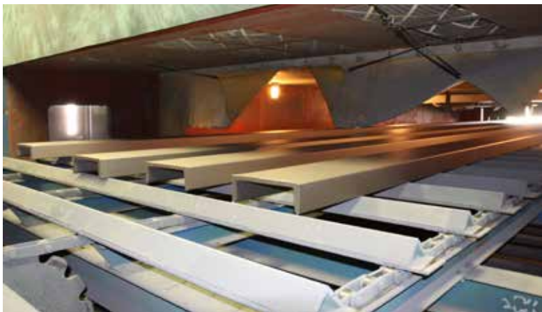
▲ The plate-processing machine can accommodate plate up to 10 ft wide and more than 60 ft long. ▼ The blast and paint line at the company's Connecticut facility.
