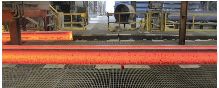
below: Beam blanks after being cut by the oxygen torch.
