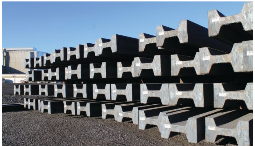
above: After cooling, beam blanks are often stored outside before they are ready to be reheated and rolled into shape.
