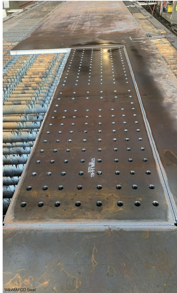
above: A single repair plate drilled and cut from a larger steel plate.
