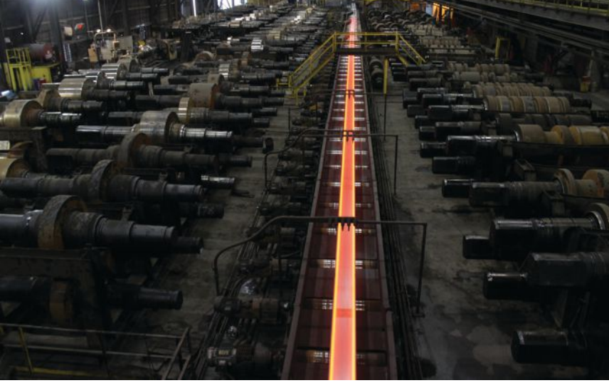
above: Steel on its way from rolling to final cutting.
