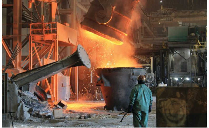
above: Transporting molten steel throughout a mini-mill.
