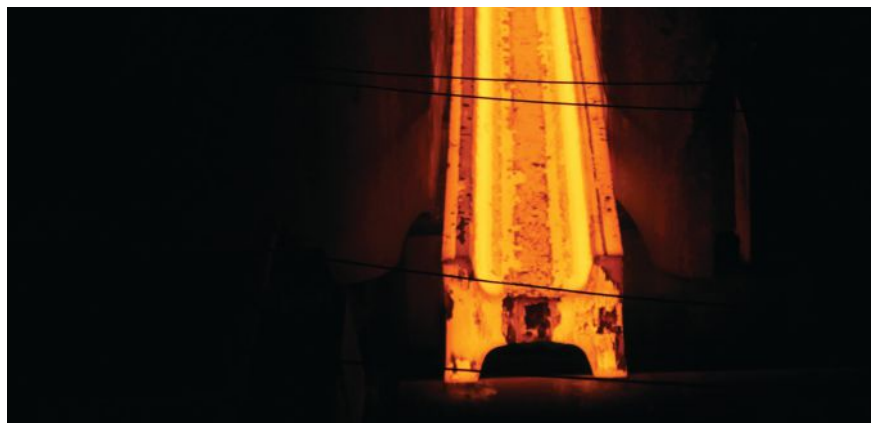
below: Steel being rolled in a universal rougher/edger mill.
