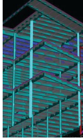
above, left, and right: The three-story structure was designed to cantilever in two different directions at each end of the building.
