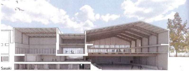
left: A cross section showing the stacking of the track and field above the ice rink.
