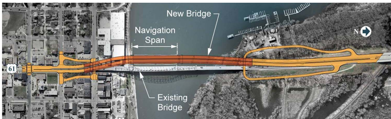
Figure 2: Site layout of new and existing structure.
