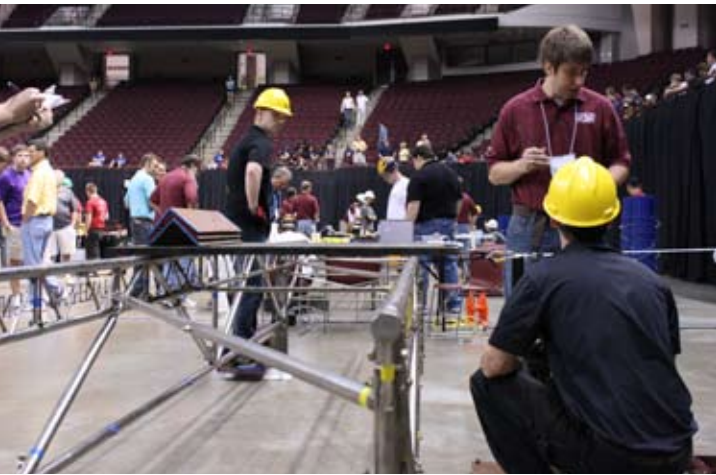
▲ Measuring the Lakehead University bridge's horizontal deflection.
